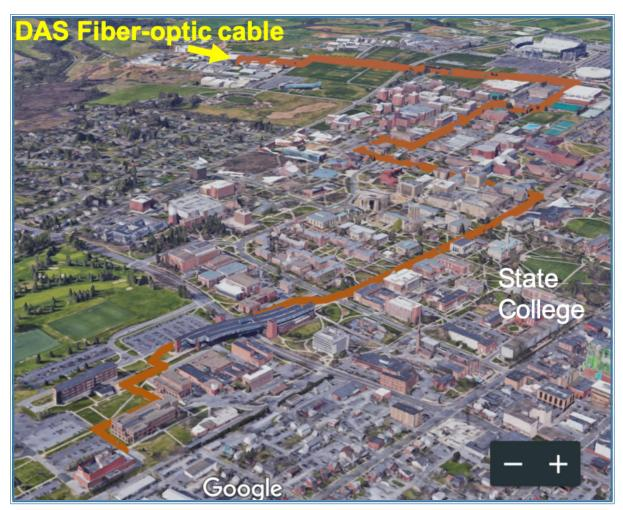
Bird's-eye view of the fiber-optic cables used for the FORESEE project in which scientists used pre-existing cables to monitor geological events
