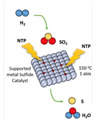
Schematic illustration of the plasma catalytic sulfur dioxide reduction with hydrogen or methane to sulfur at low temperature.
